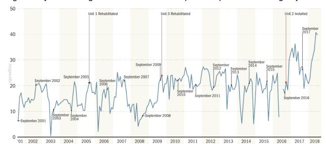
Figure 3 - Kajaki Dam Average Electric Power Generation Output from September 2001 through July 2018
