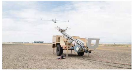
A ScanEagle unmanned aerial vehicle takes off from its pneumatic launcher. (SIGAR photo)
